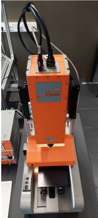
Figure 4: Hyperspectral scanner at the ITC Twente that was used to study 11 different core samples.
