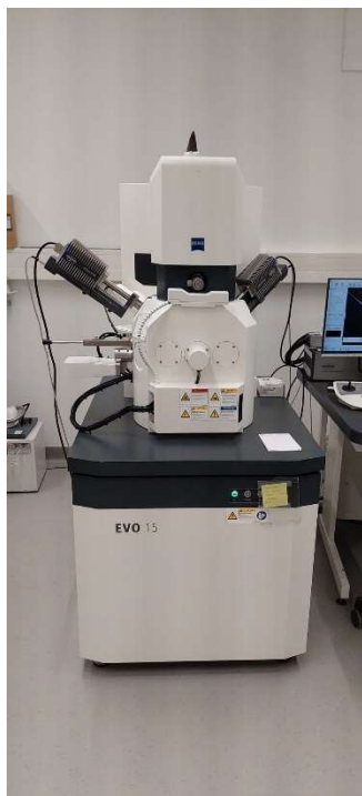
Figure 3: Scanning Electron Microscope in the UU Electron Microscopy facility that was used to study thin sections 3 and 6.
