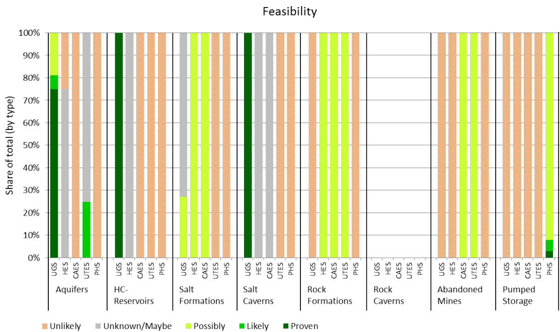
Figure 3.12-3: France - Determination of feasibility per reservoir type and technology, projected as a share of the total number of reservoirs for the given type. Classes are explained in Paragraph 1.2
