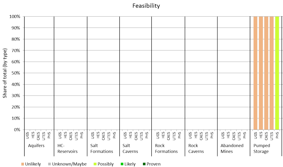
Figure 3.7-3: Cyprus - Determination of feasibility per reservoir type and technology, projected as a share of the total number of reservoirs for the given type. Classes are explained in Paragraph 1.2
