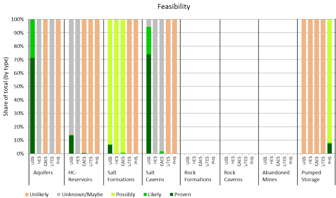
Figure 3.13-3: Germany - Determination of feasibility per reservoir type and technology, projected as a share of the total number of reservoirs for the given type. Classes are explained in Paragraph 1.2
