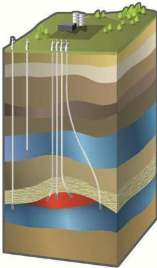
Figure 3-2: Schematic representation of storage into aquifers (blue) and (depleted) hydrocarbon reservoirs (red). The vertical scale is not consistent with reality. Source: http://www.geostockgroup.com/en/underground-storage/porous-media ).
