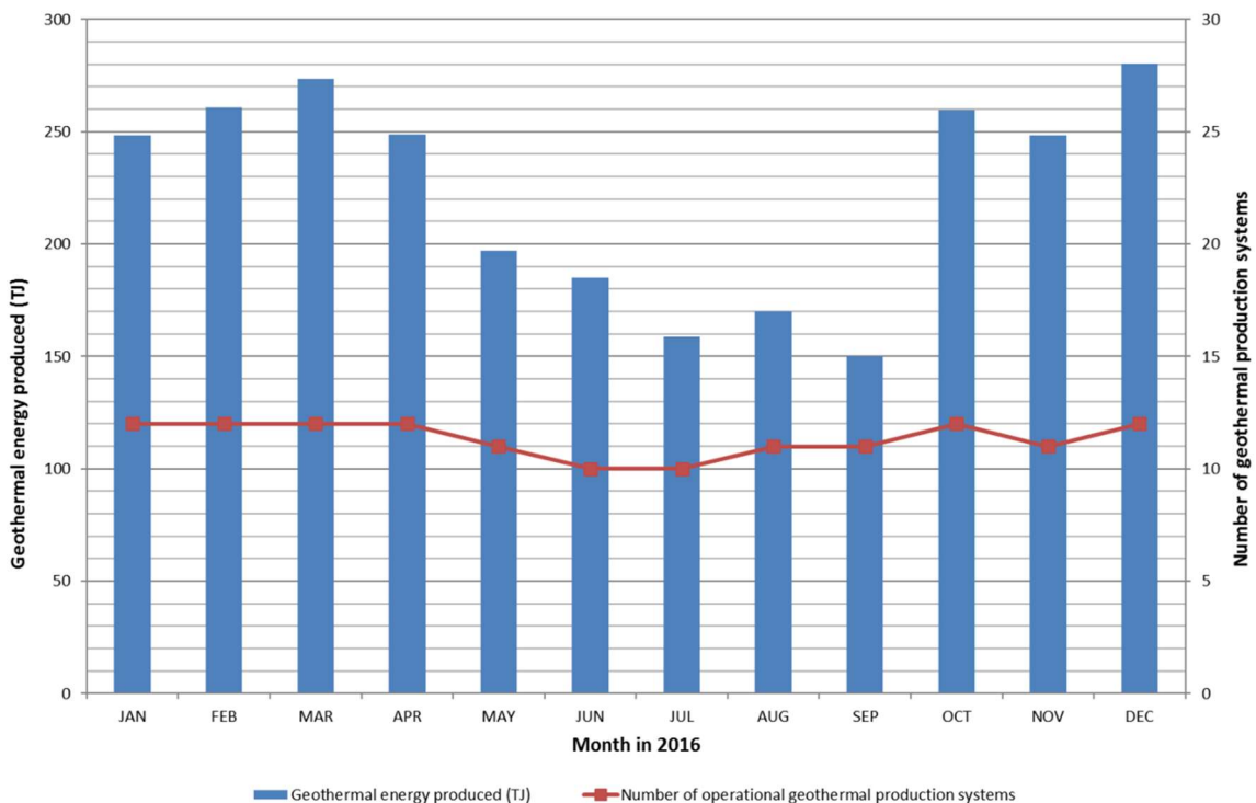
Figure 16: Monthly production of geothermal energy in tera joules and the number of geothermal energy production systems contributing to the reported production (excluding Heerlen mine water power station)
