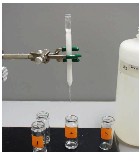
Figure A-7 Equipment for extraction and fractionation of source rock derived hydrocarbons.
