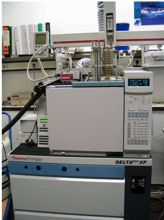
Figure A-9 The GC-IRMS system that is used for the determination of the ^{13}\text{C}/^{12}\text{C} and 2\text{H}/1\text{H} stable isotope ratios for the straight-chain n-alkanes in the source rock extracts and oil
