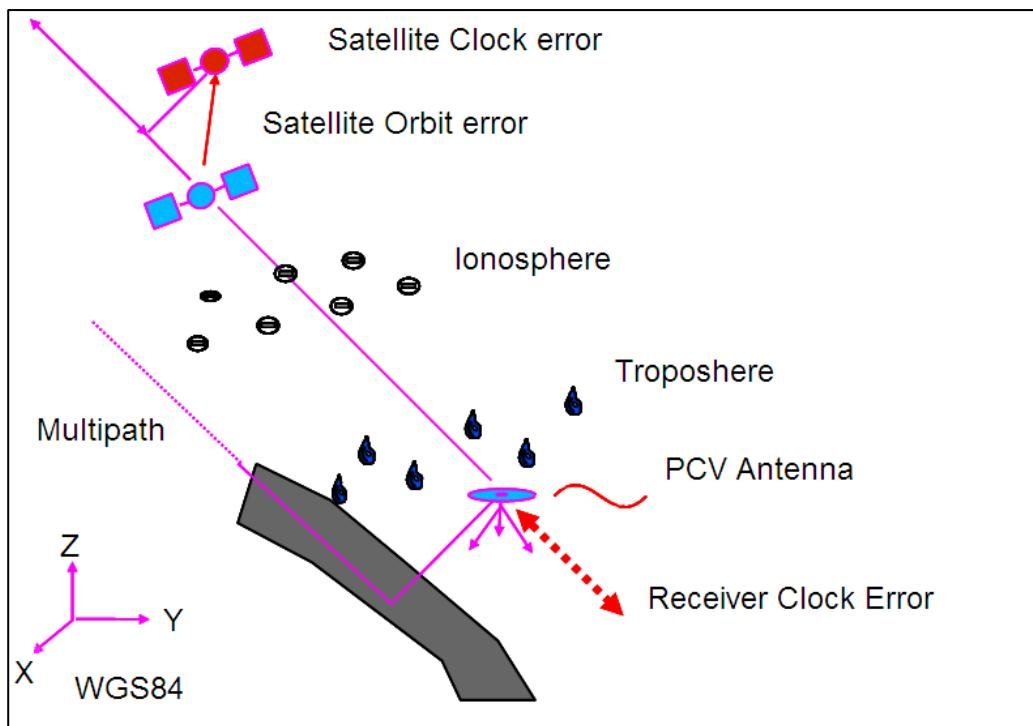
The state space modelling of GNSMART applies beforehand corrections to the GNSS observations.
